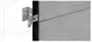
Hidden clip fastener detail Detalle de grapas invisible
